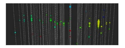
> charged current interactions:  $v_{\mu}$
